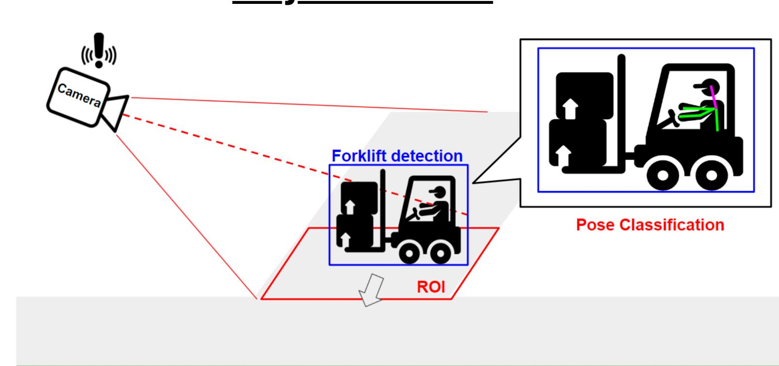
The camera was installed inside the warehouse to capture forklift activity while it passes through the intersection. Real-time images are fed via Wi-Fi to the AI station, which quickly detects and classifies any unsafe behavior of the forklift operator.
