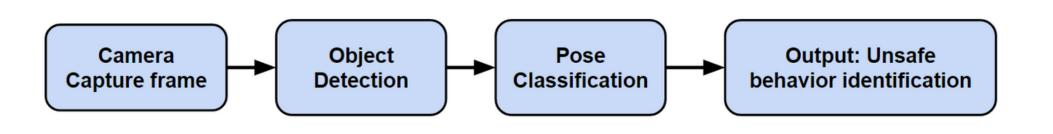
System overview: First, the input videos are from the camera. Second, the classification object forms the video. Third, estimation of human poses or actions. Finally, Estimated an unsafe behavior.
